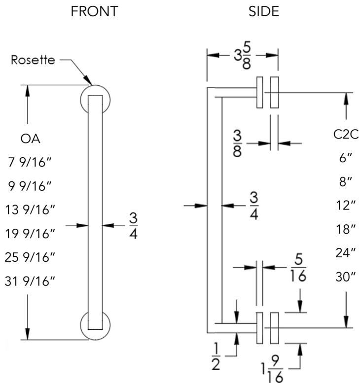
**Installation Notes:** Center to center hole drilling dimension are same as mentioned in column. Diameter of glass hole for installation is 1/2".
